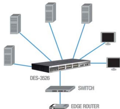
*The DES-3526 skillfully manages traffic moving through the distributed computing grid, directing all WAN packets to the gateway router. Several VLANs implemented in the grid allow for separate clusters on the same switch - increasing the bandwidth and reliability of each LAN.*
