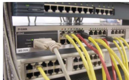
*The D-Link switch is connected to the rest of their classroom network via 100Mbps point-to-point connections. Fifteen total users - mainly students - operate the equipment.*
